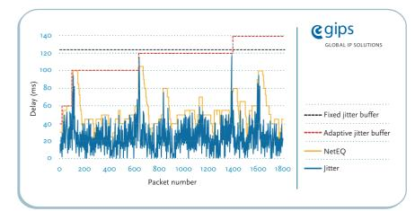
The unique non-sequential process implemented in NetEQ combines jitter buffer and error concealment in one unit. The unit detects delay variations and makes corrections before play-out and therefore produces a speech signal with highly improved sound quality. The high-resolution adaptive jitter buffer implemented in NetEQ is able to adjust quickly to the incoming jitter and operate very efficiently.
