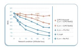
Tests of NetEQ (above) and NetEQ-wb (below) show voice quality performance over a range of network packet loss conditions. These tests were performed by Lockheed Martin Global Telecommunications (formerly Comsat), an independent test laboratory.
